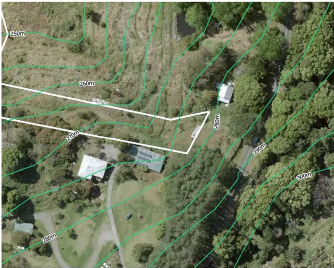
Contour survey confirming approximately 15 metre drop from road level (290M) to lot Boundary (275m)
