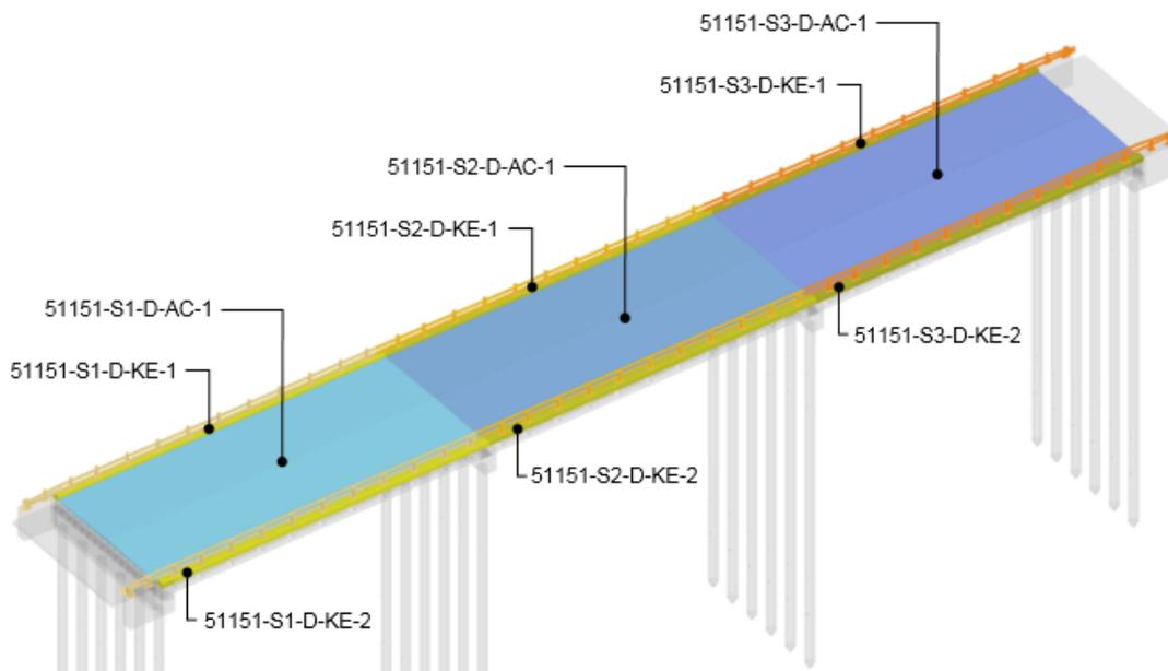
**Figure 5.2.3.2(b) – Naming convention for bridge deck objects**
