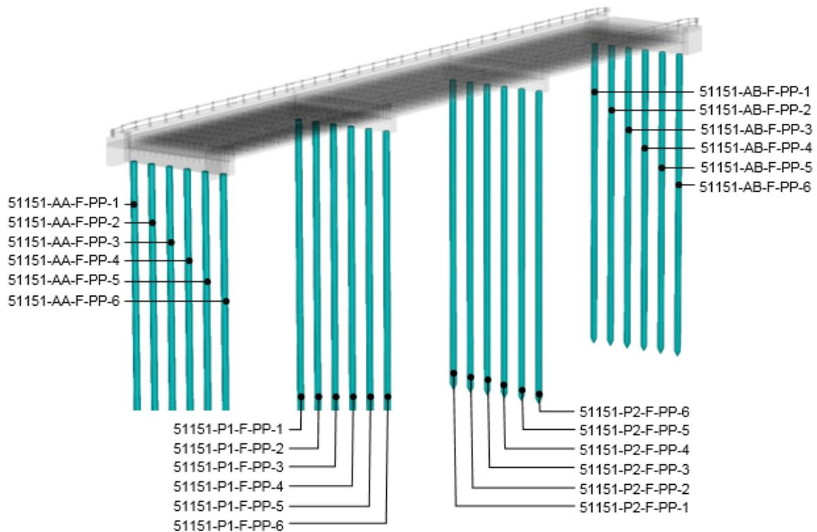
**Figure 5.2.2.1(b) – Object naming convention for piled and pad foundations**
