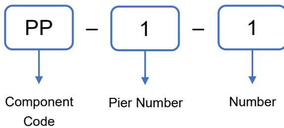
**Figure 5.1.3(d) – Short BIM object code example for a precast pile at an abutment**
