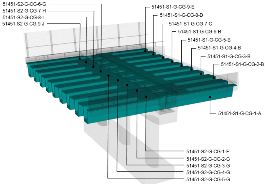
**Figure 5.2.3.1(c) – Naming convention for concrete diaphragm objects**
