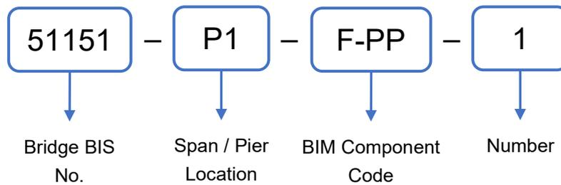
**5.1.3 Bridge BIM model object identification – short BIM object code**
