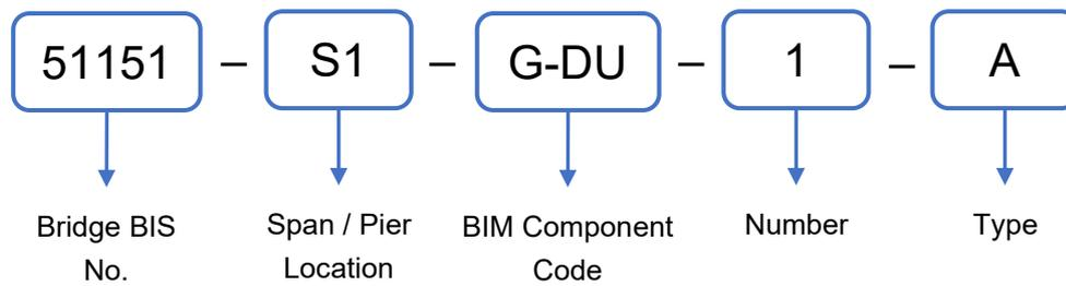
**Figure 5.1.2(c) – Full BIM object code example for a precast pile**
