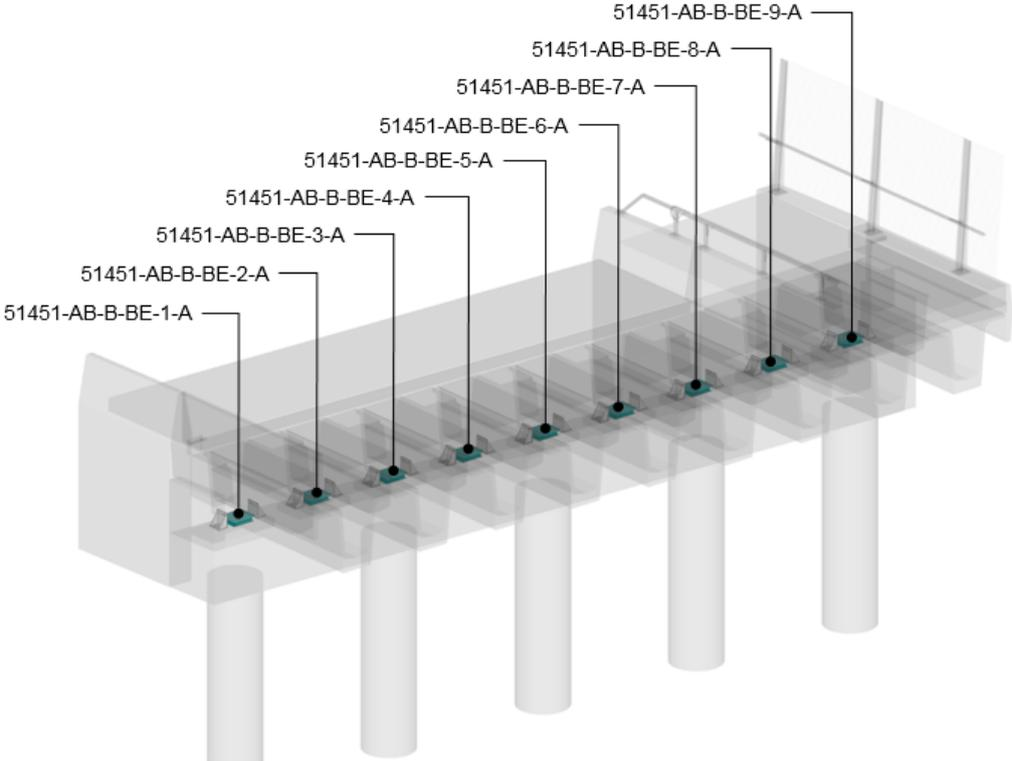
Figure 5.2.2.4(c) – Naming convention for bearing objects
