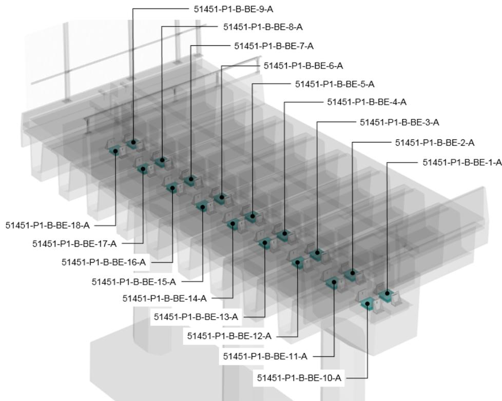
Figure 5.2.2.4(b) – Object naming convention for bearings on abutments
