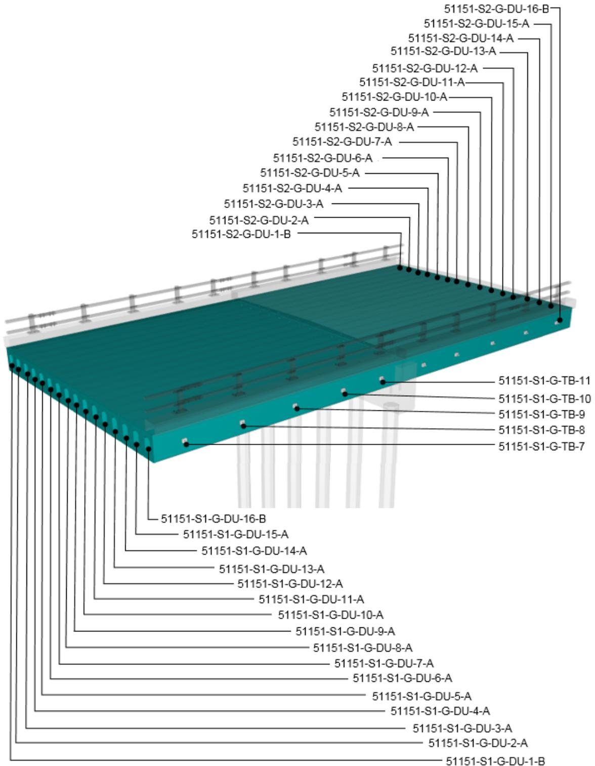
**Figure 5.2.3.1(b) – Naming convention for concrete girder (Super-T) objects**
